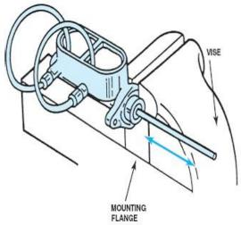
**3.** Fill the master cylinder reservoir with clean DOT 3 brake fluid from a sealed container.
