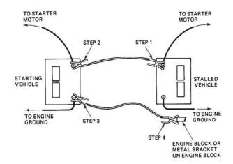
8. Disconnect the red battery cable ends from the positive terminals of the batteries.
