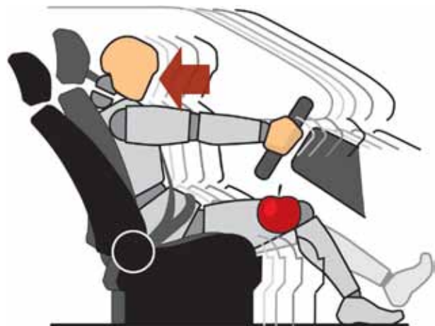
To an outside observer, the driver and car are decelerated (negatively accelerated) due to the braking force, while the apple retains its state of motion virtually force-free.
