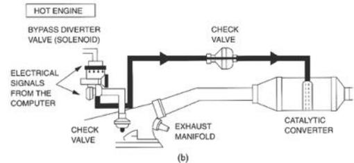
**NOTE:** A defective one-way check valve at the exhaust manifold can allow hot exhaust gases to flow past the check valve and cause damage to the switching valves, hoses or air pump itself. These exhaust gases can cause poor engine operation and stalling if drawn into the air intake system.
