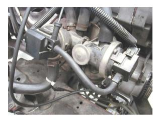
**NOTE:** A defective one-way check value at the exhaust manifold can allow hot exhaust gases to flow past the check value and cause damage to the switching values, hoses or air pump itself. These exhaust gases can cause poor engine operation and stalling if drawn into the air intake system.
