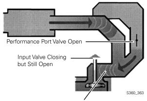
Pressure Wave for Performance Port Charges the Cylinder with Air
