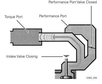
The open end of the intake duct at the torque port has the same effect on the intake wave as a solid wall has on a ball. The wave is reflected back toward the intake valve ports in the form of a high pressure wave.
