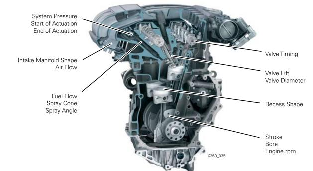
Direct gasoline injection requires precise timing of the combustion process.
