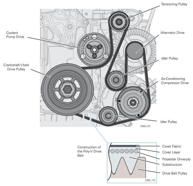
The ribbed V-belt is a single-sided poly-V belt. Even at high speed, it runs quietly and vibration-free. The belt is driven by the crankshaft through the V-belt pulley with vibration damper. The belt drives the air-conditioning compressor, the alternator and the coolant pump.
