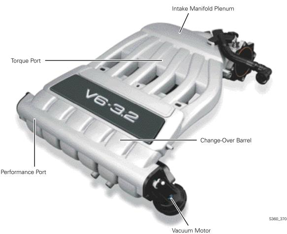
A second plenum called the performance port, which is attached to a set of short manifold ducts, joins the long intake ducts near the cylinder head. A performance port valve, similar in design to a throttle valve, separates the performance port from the short ducts.
