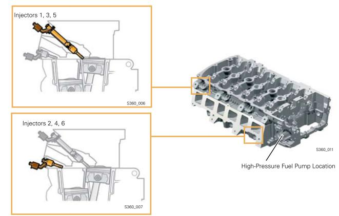
The cylinder head is made of an aluminum-siliconcopper alloy and is identical for both engines. It is a new design as a result of the direct fuel injection.
