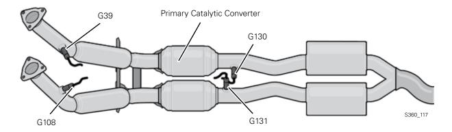
The exhaust system for the 3.2L engine has a primary ceramic catalytic converter for each cylinder bank.
