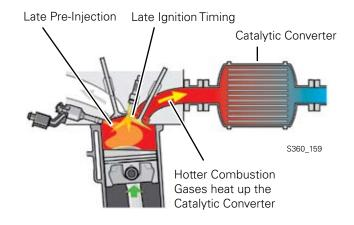
In the second injection, a small amount of fuel is additionally injected shortly before ignition Top Dead Center (TDC). The late injection increases exhaust gas temperature. The hot exhaust gas heats up the catalytic converter so that it reaches operating temperature more quickly.
