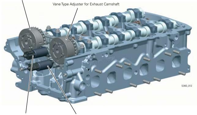
N205 Camshaft Adjustment Valve 1
