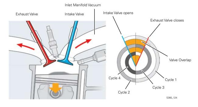
Internal exhaust gas recirculation counteracts the formation of nitrous oxides (NOx).
