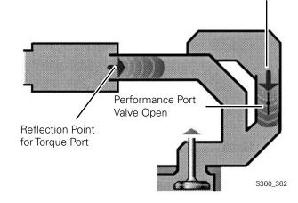
The performance port pressure wave is reflected back toward the intake valve ports, and that air is forced into the combustion chamber before the intake valves close.
