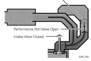
The pressure wave arriving too late from the torque port is reflected by the closed intake valves and pushes its air charge up the intake duct, filling the performance port in preparation for the next cycle.
