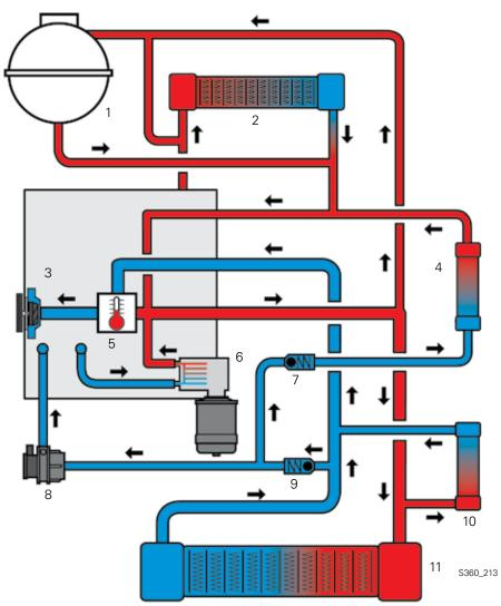
The coolant is circulated by the mechanical coolant pump. The pump is driven by the V-belt.
