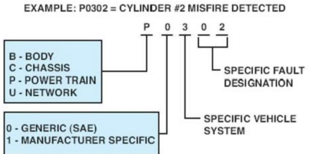
\_\_\_\_\_ 3. Retrieve and record the stored diagnostic trouble code (DTC).
