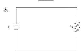
$E = I_T = 3 \text{ amperes}$   $R_T = 4 \text{ ohms}$
