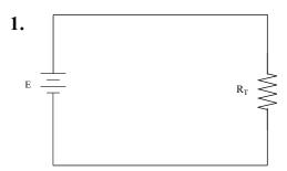
E = 12 volts  $I_T = 3 \text{ amperes}$  $R_{T=}$
