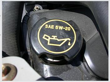
the engine was designed to use the specified viscosity. For example, the valve lifters are designed to bleed down at a certain rate and using oil that is thicker than specified can cause the valves to remain partially open when they should be closed. This can cause a misfire and poor engine operation.
