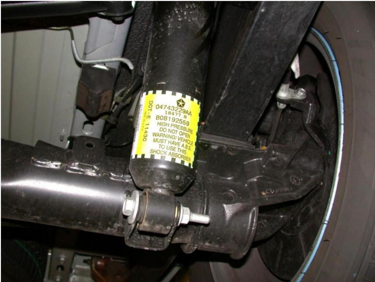
A German company, ZF Sachs, supplies a self-leveling shock absorber to several vehicle manufacturers, such as Chrysler for use on the rear of minivans, plus BMW, Saab, and Volvo. The self-leveling shocks are entirely self-contained and do not require the use of height sensors or an external air pump.
