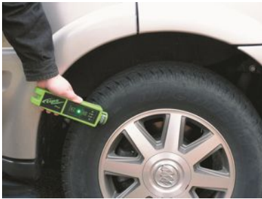
FIGURE 4.13 A typical tire-pressure monitoring system tester.
