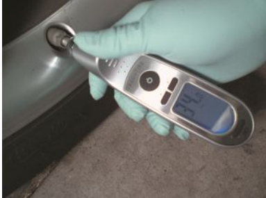
FIGURE 4.18 Always use an accurate, known-good tire-pressure gauge. Digital gauges are usually more accurate than mechanical gauges.
