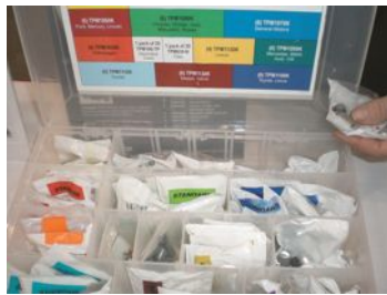
FIGURE 4.20 An assortment of service parts that include all of the parts needed to service a stem-mounted TPMS sensor being installed after removal for a tire replacement or repair.
