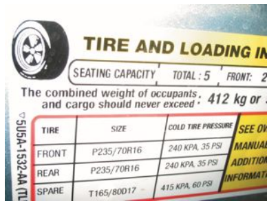
FIGURE 4.1 The tire-pressure placard (sticker) on the driver's side door or door jamb indicates the specified tire pressure.
