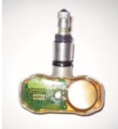
FIGURE 4.6 A clear plastic valve-stem tire-pressure monitoring sensor, showing the round battery on the right and the electronic sensor and transistor circuits on the left.
