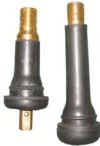
FIGURE 4.7 A conventional valve stem is on the right compared with a rubber TPMS sensor stem on the left. Notice the tapered and larger brass stem.
