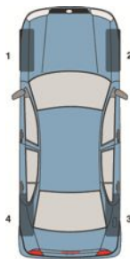
FIGURE 4.17 The sensor relearn procedure is performed in the following order after the system has been placed in learn mode: LF, RF, RR, and then LR.
