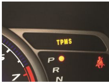
FIGURE 4.11 The TPMS warning lamp on this vehicle is a separate light from the tire icon light that warns of low tire pressure. In this case, both warning lights were on all of the time.
