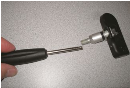
FIGURE 4.19 A clicker-type valve core tool ensures that the valve core is tightened to factory specifications.
