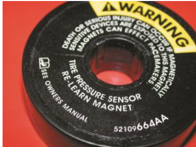
FIGURE 4.15 A magnet is placed around the valve stem to reprogram some stem-mounted tire-pressure sensors.
