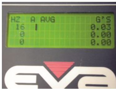
FIGURE 20.8 An electronic vibration analyzer.
