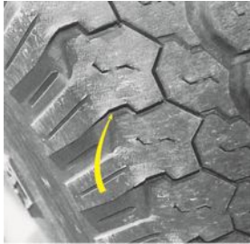
FIGURE 20.16 Tire wear caused by improper alignment or driving habits, such as high-speed cornering, can create tire noise. Notice the feather-edged outer tread blocks.
