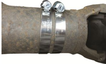
FIGURE 20.15 Two clamps were required to balance this front driveshaft of a four-wheel-drive vehicle.
