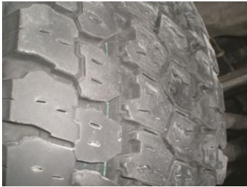
FIGURE 20.10 An out-of-balance tire showing scallops or bald spots around the tire. Even if correctly balanced, this cupped tire would create a vibration.
