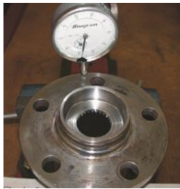
FIGURE 20.11 Another cause of a vibration that is often blamed on wheels or tires is a bent bearing hub. Use a dial indicator to check the flange for runout.
