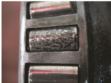
FIGURE 20.17 This bearing was found on a vehicle that had been stored over the winter. This corroded bearing produced a lot of noise and had to be replaced.
