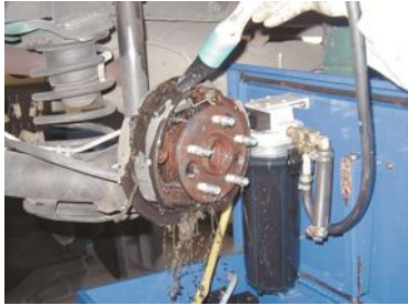
FIGURE 2.3 All brakes should be moistened with water or solvent to help prevent brake dust from becoming airborne.
