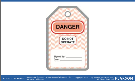
FIGURE 2.2 Tags identify that the power has been removed and service work is being done.
