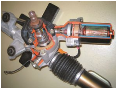
FIGURE 14.2 Honda electric power steering unit cutaway, which is an example of pinion-mounted electric power steering system.
