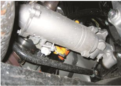
FIGURE 14.1 A rack mounted electric power steering gear on a Lexus RX 400 h taken from underneath the vehicle.
