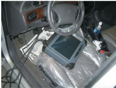
FIGURE 10.13 The use of a factory scan tool is often needed to diagnose the ESC system.
