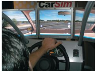
FIGURE 10.3 Using a simulator is the most cost-effective way for vehicle and aftermarket suspension manufacturers to check that the vehicle is able to perform within the FMVSS No. 126 standard for vehicle stability.
