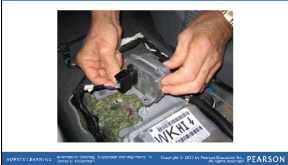
FIGURE 10.8 A lateral acceleration sensor is usually located under the center console and can be easily checked by unbolting it and turning it on its side while monitoring the sensor value using a scan tool.
