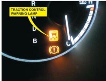
FIGURE 10.12 A traction control or low traction light on the dash is confusing to many drivers.
