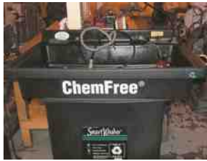
FIGURE 7.7 Using a water-based cleaning system helps reduce the hazards from using strong chemicals.
