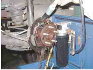
FIGURE 7.3 All brakes should be moistened with water or solvent to help prevent brake dust from becoming airborne.
