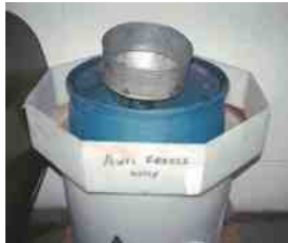
FIGURE 7.8 Used antifreeze coolant should be kept separate and stored in a leakproof container until it can be recycled or disposed of according to federal, state, and local laws. Note that the storage barrel is placed inside another container to catch any coolant that may spill out of the inside barrel.
