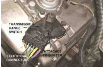
FIGURE 69.11 The transmission range (TR) switch is located on the top or side of the transmission or transaxle and is used to signal the transmission control module the position of the gear selector.
