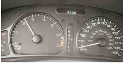
FIGURE 69.3 This 4-cylinder General Motors vehicle has a stall speed of about 2350 RPM. Notice that the gear selector is in drive and the speedometer is reading zero.
