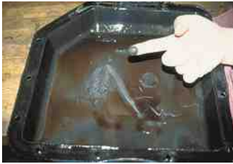
FIGURE 69.7 This is a normal amount of wear material in the bottom of an automatic transmission pan.
