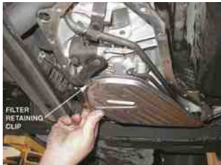
FIGURE 69.8 Always check that the filter is secured by a clip or other fastener to keep it from dropping out of location.
