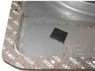
FIGURE 69.10 In this case, the cork-rubber gasket is glued to the pan and is ready to be installed. The retaining bolts need to be tightened in sequence, but be aware that overtightening will cause a leak. Also, some manufacturers recommend using only an RTV sealer, but never use an RTV sealer and a gasket together.
