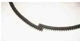
FIGURE 63.14 The starter motor will spin but the engine will not crank if the ring gear on the flywheel is broken.
