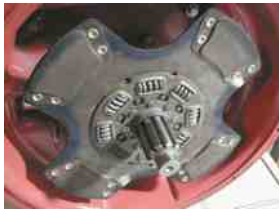
FIGURE 63.7 A racing or high-performance clutch disc lacks the features of a stock clutch disc that help provide smooth engagement.
