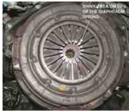
FIGURE 63.19 The release bearing rubs against the tips of the diaphragm spring.
