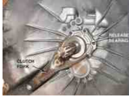
FIGURE 63.18 The clutch pedal linkage moves the clutch fork, which then applies a force against the release bearing, which then releases the clamping force the pressure plate is exerting on the clutch disc.
