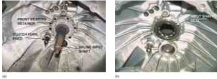
FIGURE 63.16 (a) Before replacing the clutch, the bell housing should be cleaned and the clutch fork pivot lightly lubricated. (b) The input shaft seal should also be replaced to prevent the possibility of getting transmission lubricant on the friction surfaces of the clutch.
