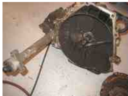
FIGURE 63.17 A transaxle assembly has been removed to replace the clutch. Note the short input shaft. This vehicle did not use a pilot bearing (bushing).
