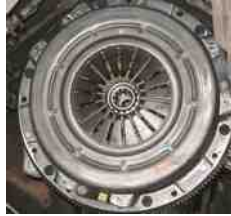
FIGURE 63.12 Typical diaphragm-style pressure plate that uses a Belleville spring.
