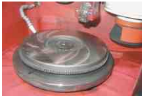
FIGURE 63.13 A flywheel after it has been machined (ground) to provide the correct surface finish for the replacement clutch disc.
