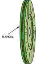
FIGURE 63.9 A marcel is a wavy spring that is placed between the two friction surfaces to cushion the clutch engagement.
