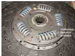
FIGURE 63.8 A typical stock clutch friction disc that uses coil spring torsional dampers.
