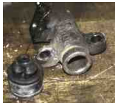
FIGURE 63.20 The clutch slave cylinder is often corroded because of moisture absorbed by the brake fluid used in the hydraulic clutch. This slave cylinder was disassembled to see if it could be overhauled rather than replaced.
