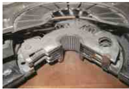
FIGURE 63.10 Cutaway of the center section of a clutch plate showing the various layers of steel plates used in the construction.
