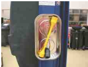
FIGURE 6.7 A magnetic tray is a helpful item to keep tools needed up where they can be easily reached without having to bend over saving time and energy over the course of a long day in the shop.
