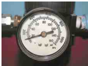
FIGURE 6.11 The air pressure going to the nozzle should be reduced to 30 PSI or less.
