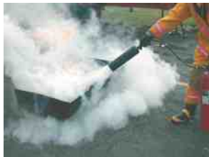
FIGURE 6.13 A CO2 fire extinguisher being used on a fire set in an open steel drum during a demonstration at a fire department training center.
