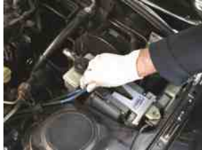
FIGURE 6.3 Protective gloves such as these vinyl gloves are available in several sizes. Select the size that allows the gloves to fit snugly. Vinyl gloves last a long time and often can be worn all day to help protect your hands from dirt and possible hazardous materials.
