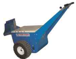
FIGURE 6.8 An electric pusher used to push vehicles into or around the shop.
