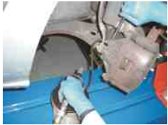
FIGURE 56.7 Using a compressed air-powered vacuum bleeder.
