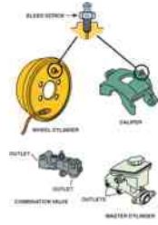
FIGURE 56.3 Typical bleeder locations. Note that the combination valve and master cylinder shown do not have bleeder valves; therefore, bleeding is accomplished by loosening the brake line at the outlet ports.
