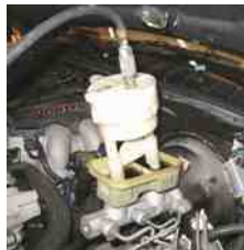
FIGURE 56.11 Brake fluid under pressure from the power bleeder is applied to the top of the master cylinder. It is very important that the proper adapter be used for the master cylinder. Failure to use the correct adapter or failure to release the pressure on the brake fluid before removing the adapter can cause fluid to escape under pressure.
