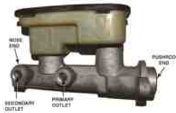
FIGURE 54.12 The primary outlet is the outlet closest to the pushrod end of the master cylinder and the secondary outlet is closest to the nose end of the master cylinder.
