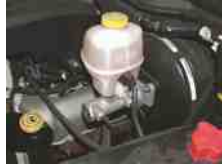
FIGURE 54.3 Master cylinder with brake fluid level at the "max" (maximum) line.
