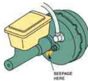
FIGURE 54.17 Some seepage is normal when a trace of fluid appears on the vacuum booster shell. Excessive leakage, however, indicates a leaking secondary (and) seal.
