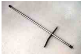
FIGURE 54.16 A brake pedal depressor like this can be used during brake service to block the flow of brake fluid from the master cylinder during service work on the hydraulic system.
