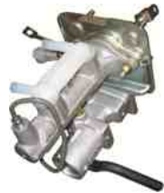
FIGURE 53.11 A master cylinder from a Toyota Highlander hybrid electric vehicle.
