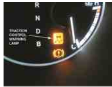
FIGURE 53.10 A traction control or low traction light on the dash is confusing to many drivers. When the lamp is on or flashing, it indicates that a low traction condition has been determined and the traction control system is working to restore traction. A flashing traction dash light does not indicate a fault.
