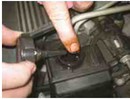
FIGURE 51.23 A check of the power steering fluid should include inspecting not only the level but the condition and color of the fluid, which could indicate a possible problem with other components in the steering system.
