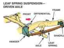
FIGURE 49.4 A typical rear-wheel-drive pickup truck rear suspension equipped with leaf springs. This type of arrangement is called a Hotchkiss drive and the drivetrain forces are controlled by the rear suspension components.
