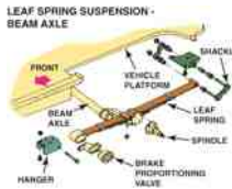
FIGURE 49.5 An exploded view of a beam axle with multileaf springs.
