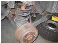
FIGURE 49.20 The shock absorber needs to be disconnected before removing the coil spring. Installation is the reverse of removal procedure.
