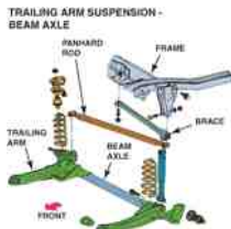
FIGURE 49.8 A typical beam axle rear suspension, which uses trailing arms and coil springs along with a track rod, also called a Panhard rod, to control side-to-side axle movement.
