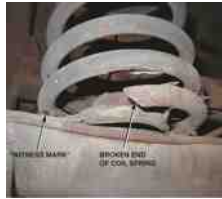
FIGURE 49.19 A broken spring was discovered during a routine under-vehicle visual inspection. Notice the witness marks that show that the spring coils have been hitting each other.
