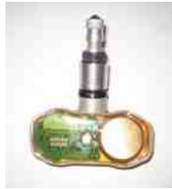
FIGURE 46.5 A clear plastic valve-stem tire-pressure monitoring sensor, showing the round battery on the right and the electronic sensor and transistor circuits on the left.
