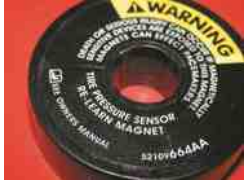
FIGURE 46.13 A magnet is placed around the valve stem to reprogram some stem-mounted tire-pressure sensors.
