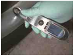
FIGURE 46.14 Always use an accurate, known-good tirepressure gauge. Digital gauges are usually more accurate than mechanical gauges.
