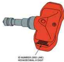
FIGURE 46.12 When replacing a TPMS sensor, be sure to record the sensor ID because this needs to be entered into the system through the use of a tester or scan tool.
