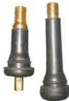
FIGURE 46.6 A conventional valve stem is on the right compared with a rubber TPMS sensor stem on the left. Notice the tapered and larger brass stem. The rubber TPMS sensor also uses a longer cap that makes it easy for a technician to spot that this is not a conventional rubber valve stem.
