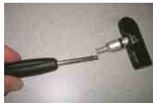
FIGURE 46.15 A clicker-type valve core tool ensures that the valve core is tightened to factory specifications.
