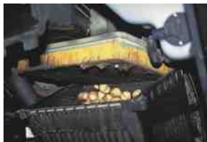
FIGURE 44.5 This is what was found when removing an air filter from a vehicle that had a lack-of-power concern. Obviously, the nuts were deposited by squirrels or some other animal, blocking a lot of the airflow into the engine.
