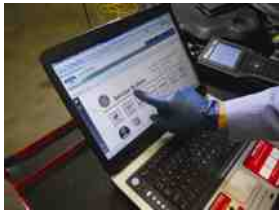
FIGURE 44.7 After checking for stored diagnostic trouble codes (DTCs), the wise technician checks service information for any technical service bulletins that may relate to the vehicle being serviced.
