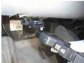
FIGURE 44.4 Connecting a scan tool to the data link connector (DLC) located under the dash on this vehicle.
