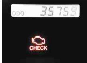
FIGURE 44.3 A typical malfunction indicator lamp (MIL) often labeled "check engine" or "service engine soon" (SES).
