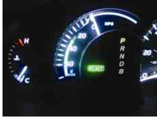
FIGURE 43.6 If the "Ready" light is on, then the gasoline engine can start at any time and the vehicle can be driven in electric mode for a short distance and limited speed.
