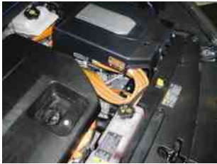
FIGURE 43.4 Orange-colored cable under the hood means that the vehicle is a hybrid or an electric vehicle that uses high-voltage components and circuits.
