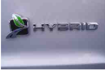
FIGURE 43.3 Look for an emblem that says "Hybrid" on the front, side, or rear of the vehicle
