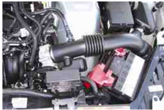
FIGURE 43.10 This 12-volt battery under the hood on a Ford Fusion hybrid is a flooded cell-type auxiliary battery.
