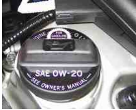
FIGURE 43.9 Always use the specified viscosity of oil in a hybrid electric vehicle not only for best fuel economy but also because of the need for fast lubrication due to the engine (idle)stop feature.
