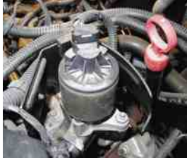
FIGURE 42.3 A General Motors electronic EGR valve.
