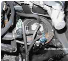
FIGURE 42.11 A charcoal canister can be located under the hood or underneath the vehicle.
