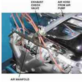
FIGURE 42.7 The external air manifold and exhaust check valve on a restored muscle car engine.
