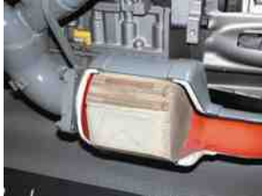
FIGURE 42.9 Most catalytic converters are located as close to the exhaust manifold as possible, as seen in this display of a Chevrolet Corvette.
