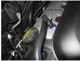
FIGURE 42.4 A PCV valve and hose on a Ford 5.0-liter V-8. Many are hard to see as they are hidden from view under plastic covers.
