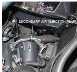
FIGURE 42.8 A typical electric motor-driven SAI pump. This unit is on a Chevrolet Corvette and only works when the engine is cold.
