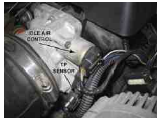
FIGURE 41.7 An idle control unit has four wires and it uses a reversible stepper motor to regulate the amount of air bypassing the throttle plate.
