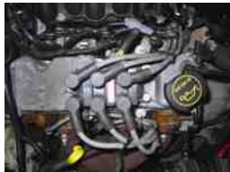
FIGURE 39.4 A Ford V-6 engine that uses a waste-sparktype ignition system. Note that each of the three coils has two spark plug wires. Both the cylinders fire at the same time.
