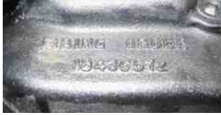
FIGURE 39.3 The firing order is cast or stamped on the intake manifold on most engines that have a distributor ignition.
