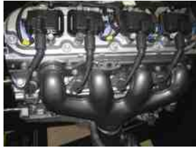
FIGURE 39.6 This General Motors V-8 engine is equipped with a coil-near-plug ignition. Each cylinder has a coil and uses a short spark plug wire from the coil to the spark plug.
