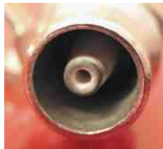
FIGURE 39.8 A close-up showing the recessed center electrode on a spark tester. It is recessed 3/8 in. into the shell and the spark must then jump another 3/8 in. to the shell for a total gap of 3/4 in.
