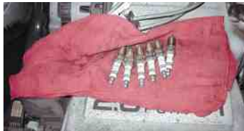
FIGURE 39.14 When removing spark plugs, it is wise to arrange them so that they can be compared and any problem can be identified with a particular cylinder.
