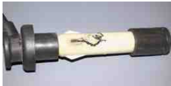
FIGURE 39.11 This spark plug boot on an overhead camshaft engine has been arcing to the valve cover causing a misfire to occur.
