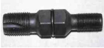
FIGURE 39.15 A spark plug thread chaser is a low-cost tool that hopefully will not be used often, but is necessary in order to clean the threads before installing new spark plugs.
