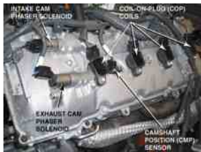
FIGURE 39.5 An overhead camshaft engine equipped with variable valve timing on both the intake and exhaust camshafts and the coil-on-plug ignition.
