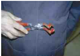
FIGURE 39.10 Spark plug wire boot pliers are a handy addition to any tool box.
