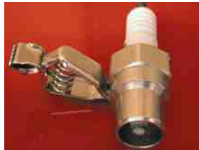
FIGURE 39.7 A spark tester looks like a regular spark plug with an alligator clip attached to the shell. This tester has a specified gap that requires at least 25,000 volts (25 kV) to fire.
