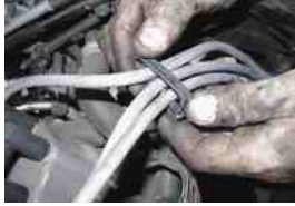
FIGURE 39.9 Spark plug wires carry high-voltage pulses from the ignition coil or distributor to the spark plugs. Always take the time to install spark plug wires back into the original holding brackets (wiring combs).
