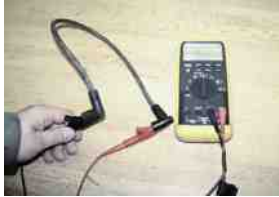
FIGURE 39.12 Measuring the resistance of a spark plug wire with a multimeter set to the ohms position. The reading of 16.03 k \Omega (16,030 ohms) is okay because the wire is about 2-ft long. Maximum allowable resistance for a spark plug wire this long would be 20 k \Omega (20,000 ohms).
