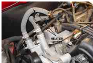
FIGURE 38.5 Heater hoses are the smaller coolant hoses that run from and back to the engine.
