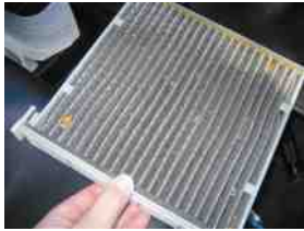
FIGURE 38.4 A typical cabin filter being removed from behind the glove compartment.
