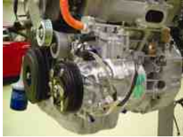
FIGURE 38.9 Hybrid electric vehicle AC compressor. Note that this unit is primarily belt-driven but has a high-voltage electric motor built in to allow the AC system operation during idle stop.
