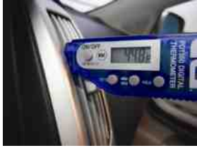
FIGURE 38.3 An air-conditioning thermometer being used to check the discharge temperature at the center vents.
