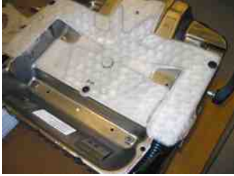
FIGURE 36.21 A gel-filled (bladder-type) occupant detection sensor showing the pressure sensor and wiring.
