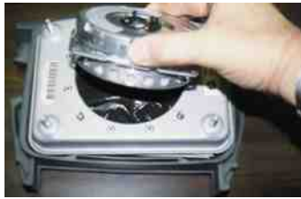
FIGURE 36.7 The inflator module is being removed from the airbag housing. The squib, inside the inflator module, is the heating element that ignites the pyrotechnic gas generator that rapidly produces nitrogen gas to fill the airbag.
