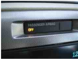
FIGURE 36.19 A dash warning lamp will light if the passenger side airbag is off because no passenger was detected by the seat sensor.
