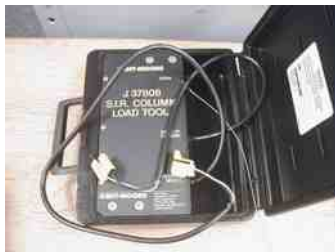
FIGURE 36.14 An airbag diagnostic tester. Included in the plastic box are electrical connectors and a load tool that substitutes for the inflator module during troubleshooting.
