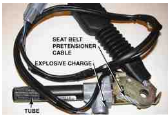
FIGURE 36.4 A small explosive charge in the pretensioner forces the end of the seat belt down the tube, which removes any slack in the seat belt.
