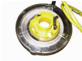
FIGURE 36.17 An airbag clockspring showing the flat conductor wire. It must be properly positioned to ensure proper operation.
