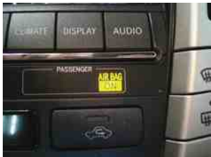
FIGURE 36.20 The passenger side airbag "on" lamp will light if a passenger is detected on the passenger seat.
