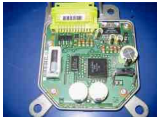
FIGURE 36.11 A sensing and diagnostic module that includes an accelerometer.
