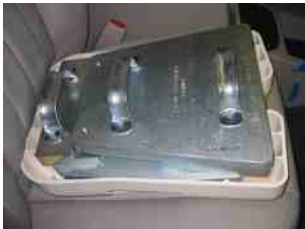
FIGURE 36.23 A test weight is used to calibrate the occupant detection system on a Chrysler vehicle.
