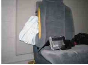
FIGURE 36.24 A typical seat (side) airbag that deploys from the side of the seat.
