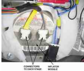
FIGURE 36.12 A driver's side airbag showing two inflator connectors. One is for the lower force inflator and the other is for the higher force inflator. Either can be ignited or both at the same time if the deceleration sensor detects a severe impact.
