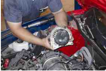
FIGURE 31.14 Replacing an alternator is not always as easy as it is from a Buick with a 3800 V-6, where the alternator is easy to access. Many alternators are difficult to access, and require the removal of other components.
