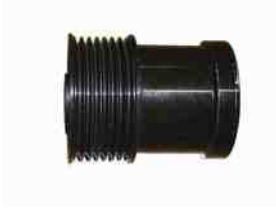
FIGURE 31.8 This overrunning alternator dampener (OAD) is longer than an overrunning alternator pulley (OAP) because it contains a dampener spring as well as a one-way clutch. Be sure to check that it locks in one direction.
