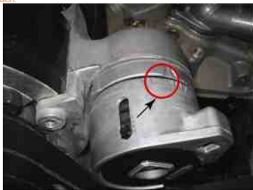
FIGURE 31.7 Check service information for the exact marks where the tensioner should be located for proper belt tension.
