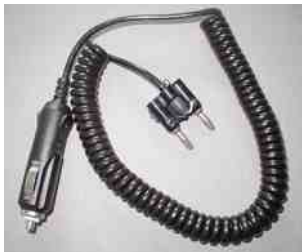
FIGURE 31.10 Charging system voltage can be easily checked at the lighter plug by connecting a lighter plug to the voltmeter through a double banana plug.
