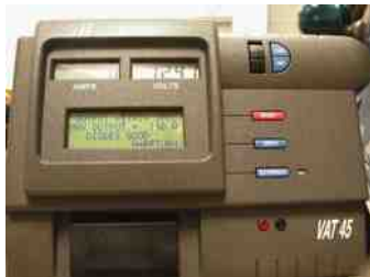
FIGURE 31.13 A typical tester used to test batteries as well as the cranking and charging system. Always follow the operating instructions.
