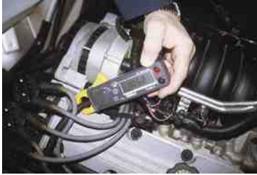
FIGURE 31.11 A mini clamp-on meter can be used to measure alternator output as shown here (105.2 amperes). Then the meter can be used to check AC current ripple by selecting AC amps on the rotary dial. AC ripple current should be less than 10% of the DC current output.
