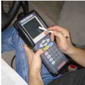
FIGURE 31.4 A scan tool can be used to diagnose charging system problems.
