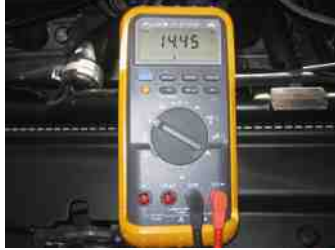
FIGURE 31.3 The digital multimeter should be set to read DC volts, with the red lead connected to the positive (+) battery terminal and the black meter lead connected to the negative (-) battery terminal.
