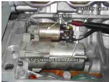
FIGURE 30.10 The starter is located under the intake manifold on this Cadillac North star engine.
