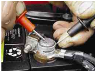
FIGURE 30.8 To test the voltage drop of the battery cable connection, place one voltmeter lead on the battery terminal and the other voltmeter lead on the cable end and crank the engine. The voltmeter will read the difference in voltage between the two leads, which should not exceed 0.20 volt (200 millivolts).
