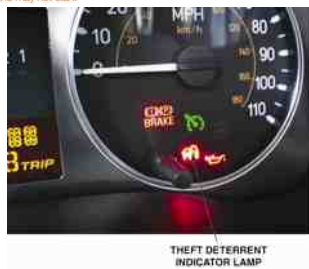
FIGURE 30.5 A theft deterrent indicator lamp of the dash. A flashing lamp usually indicates a fault in the system, and the engine may not start.
