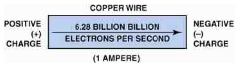
FIGURE 23.11 One ampere is the movement of 1 coulomb (6.28 billion electrons) past a point in 1 second.
