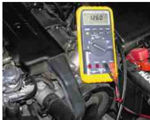
FIGURE 23.14 This digital multimeter set to read DC volts is being used to test the voltage of a vehicle battery. Most multimeters can also measure resistance (ohms) and current flow (amperes).
