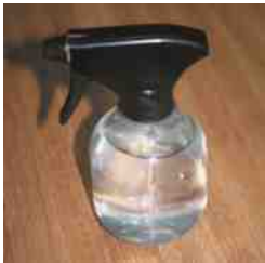
FIGURE 17.21 A water spray bottle is an excellent diagnostic tool to help determine if the noise is due to an accessory drive belt. If the noise goes away when the belt is sprayed with a mist of water, then the belt is the cause.
