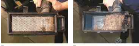
FIGURE 17.6 (a) A typical dirty air filter. (b) Always check the inlet passage leading to the air filter for debris that can reduce airflow to the engine.
