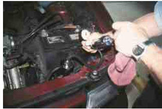
FIGURE 17.15 Pressure testing the cooling system. A typical hand-operated pressure tester applies pressure equal to the radiator cap pressure. The pressure should hold; if it drops, this indicates a leak somewhere in the cooling system. An adapter is used to attach the pump to the cap to determine if the radiator can hold pressure, and release it when pressure rises above its maximum rated pressure setting.
