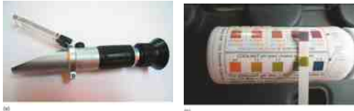
FIGURE 17.14 (a) A refractometer is used to measure the freezing point of coolant. A drop of coolant is added to a viewing screen, the lid is closed, and then held up to the light to view the display on the tool. (b) The use of test strips is a convenient and cost-effective method to check coolant condition and freezing temperature.
