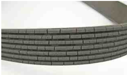
FIGURE 17.18 A typical worn serpentine accessory drive belt. Newer belts made from ethylene propylene diene monomer (EPDM) do not crack like older belts that were made from neoprene rubber.
