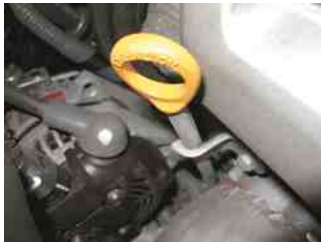
FIGURE 17.10 A typical oil level indicator (dipstick).
