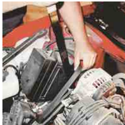
FIGURE 17.17 A special tool is useful when installing a new accessory drive belt. The long-handled wrench fits in a hole of the belt tensioner.
