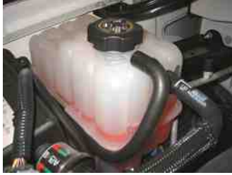
FIGURE 17.13 Visually check the level and color of coolant in the coolant recovery or surge tank.
