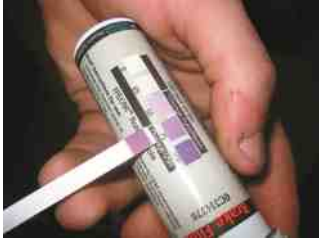
FIGURE 17.9 Brake fluid test strips are a convenient and easy-to-use method to determine if the brake fluid needs to be replaced.
