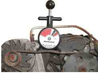
FIGURE 17.19 A belt tension gauge displays the belt tension in pounds of force.
