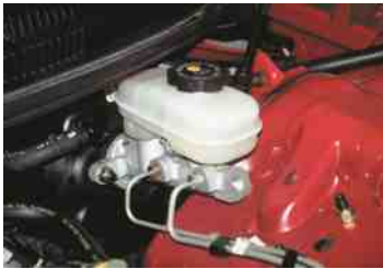
FIGURE 17.7 A master cylinder with a transparent reservoir. The brake fluid level should be between the MAX and the MIN levels as marked on the reservoir.
