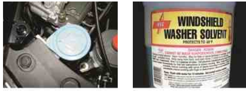
FIGURE 17.4 (a) The windshield wiper fluid reservoir cap is usually labeled with a symbol showing a windshield washer. (b) Use only the recommended washer fluid. Never use antifreeze in the windshield washer reservoir.
