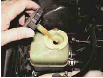
FIGURE 17.22 Most vehicles use a combination filler cap and level indicator (dipstick) that shows the level of power steering fluid in the reservoir.
