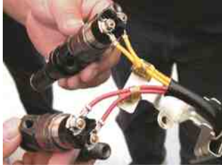
FIGURE 16.12 Typical computer-controlled diesel engine fuel injectors.
