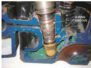
FIGURE 16.11 A HEUI injector from a Ford Power Stroke diesel engine. The O-ring grooves indicate the location of the O-rings that seal the fuel section of the injector from coolant and from the engine oil.
