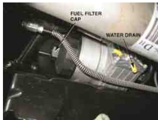
FIGURE 16.7 A fuel filter attached to the frame rail on a Ford pickup truck equipped with a diesel engine. When the "water in fuel" warning lamp comes on, the water that is trapped in the filter-water separator assembly can be drained from the unit.
