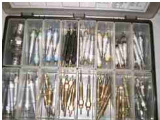
FIGURE 16.14 A glow plug assortment showing the various types and sizes of glow plugs used. Always use the specified glow plugs.
