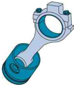
FIGURE 16.4 A rod/piston assembly from a 5.9 liter Cummins diesel engine used in a Dodge pickup truck.
