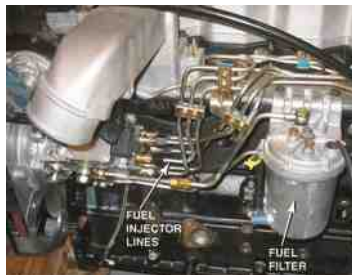
FIGURE 16.8 A typical distributor-type diesel injection pump showing the pump, lines, and fuel filter.
