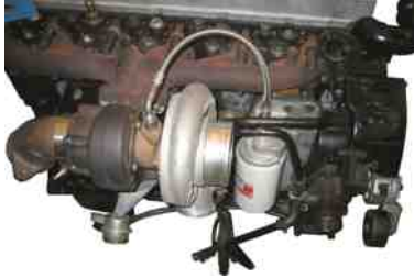
FIGURE 16.15 A Cummins diesel turbocharger is used to increase the power and torque of the engine.
