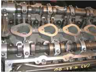
FIGURE 15.14 A DOHC engine uses a camshaft for the intake valve and a separate camshaft for the exhaust valves in each cylinder head.
