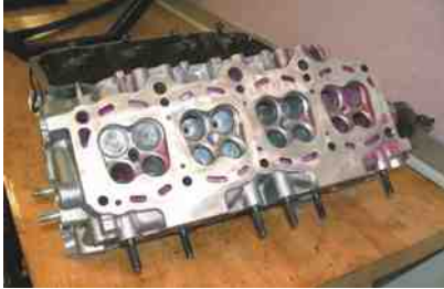
FIGURE 15.3 A cylinder head with four valves per cylinder, two intake valves (larger) and two exhaust valves (smaller).
