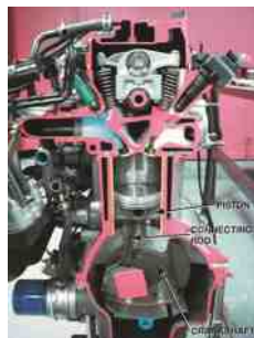
FIGURE 15.7 Cutaway of an engine showing the cylinder, piston, connecting rod, and crankshaft.
