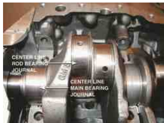
FIGURE 15.19 The distance between the centerline of the main bearing journal and the centerline of the connecting rod journal determines the stroke of the engine. This photo is a little unusual because it shows a V-6 with a splayed crankshaft used to even out the impulses on a 90° V-6 engine design.
