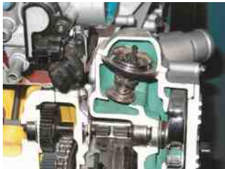
FIGURE 15.4 The coolant temperature is controlled by the thermostat, which opens and allows coolant to flow to the radiator when the temperature reaches the rated temperature of the thermostat.
