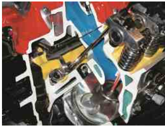
FIGURE 15.12 Cutaway of an overhead valve (OHV) V-8 engine showing the lifters, pushrods, roller rocker arms, and valves.
