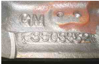
FIGURE 14.5 Engine block identification number cast into the block is used for identification.
