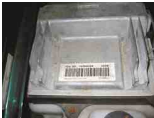
FIGURE 14.4 A typical computer calibration sticker on the case of the controller. The information on the sticker is often needed when ordering parts or a replacement controller.
