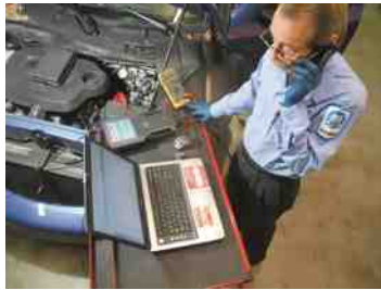
FIGURE 13.4 Whenever calling a hot line service be sure that you have all of the vehicle information ready and are prepared to give answers regarding voltage readings or scan tool data when talking to the vehicle specialist.
