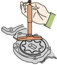
FIGURE 12.21 A depth micrometer being used to measure the height of the rotor of an oil pump from the surface of the housing.
