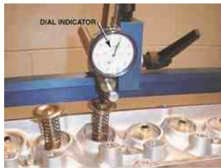
FIGURE 12.19 A dial indicator is used to measure valve lift during flow testing of a high-performance cylinder head.
