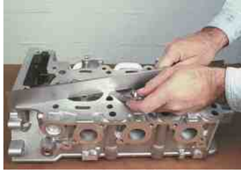
FIGURE 12.18 A straightedge is used with a feeler gauge to determine if a cylinder head is warped or twisted.
