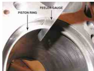
FIGURE 12.17 A feeler gauge, also called a thickness gauge, is used to measure the small clearances such as the end gap of a piston ring.
