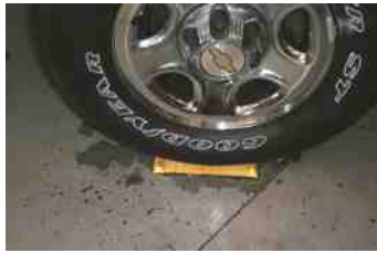
UNFIGURE 11.02 Most vehicles will be correctly positioned when the left front tire is centered on the tire pad.
