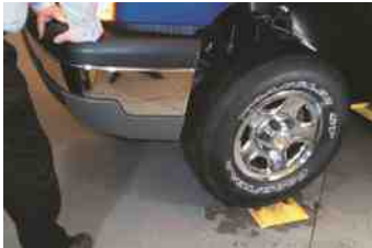
UNFIGURE 11.09 With the vehicle raised one foot (30 cm) off the ground, push down on the vehicle to check to see if it is stable on the pads. If the vehicle rocks, lower the vehicle and reset the pads. The vehicle can be raised to any desired working level. Be sure the safety is engaged before working on or under the vehicle.
