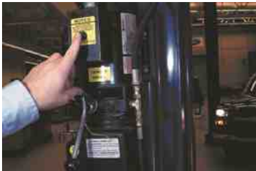
UNFIGURE 11.08 After being sure all pads are correctly positioned, use the hoist controls to raise the vehicle.
