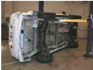
FIGURE 11.5 This training vehicle fell from the hoist when the pads were not set correctly. No one was hurt, but the vehicle was damaged.
