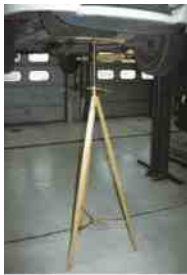
FIGURE 11.4 (a) Tall safety stands can be used to provide additional support for a vehicle while on a hoist. (b) A block of wood should be used to avoid the possibility of doing damage to components supported by the stand.
