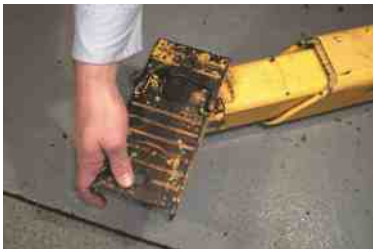
UNFIGURE 11.03 The arms can be moved in and out and most pads can be rotated to allow for many different types of vehicle construction.
