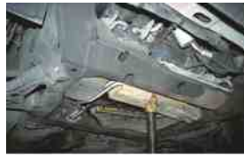
FIGURE 11.4 (a) Tall safety stands can be used to provide additional support for a vehicle while on a hoist. (b) A block of wood should be used to avoid the possibility of doing damage to components supported by the stand.
