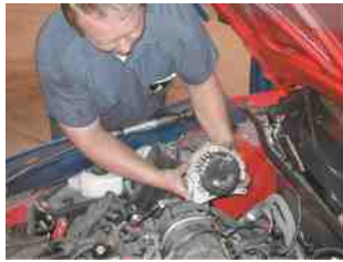
FIGURE 1.10 The alternator is in the heart of the electrical system.
