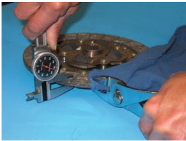
Figure 5-8 The thickness of the clutch disc facing can be measured using a vernier caliper.
