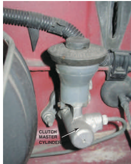
Figure 5-2 A typical clutch master cylinder and reservoir mounted on the bulkhead on the driver's side of the vehicle.
