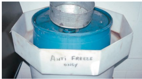
Figure 2-8 Used antifreeze coolant should be kept separate and stored in a leak-proof container until it can be recycled or disposed of according to federal, state, and local laws. Note that the storage barrel is placed inside another container to catch any coolant that may spill out of the inside barrel.
