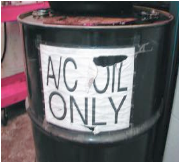
Figure 2–10 Air-conditioning refrigerant oil must be kept separated from other oils because it contains traces of refrigerant and must be treated as hazardous waste.
