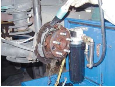
FIGURE 2-3 All brakes should be moistened with water or solvent to help prevent brake dust from becoming airborne.
