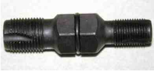
FIGURE 30.15 A spark plug thread chaser is a low-cost tool that hopefully will not be used often, but is necessary in order to clean the threads before installing new spark plugs.
