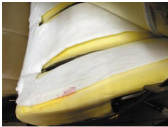
FIGURE 9-6 The heating element of a heated seat is a replaceable part, but service requires that the upholstery be removed. The yellow part is the seat foam material and the entire white cover is the replaceable heating element. This is then covered by the seat material.
