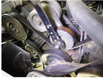
FIGURE 9-4 A special wrench being used to remove the tension from the accessory drive belt so it can be removed.
