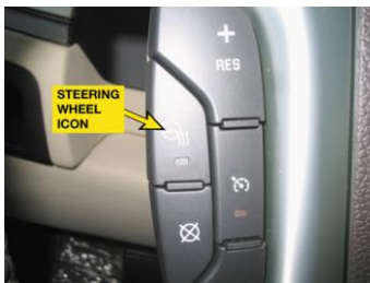
FIGURE 9-8 The heated steering wheel is controlled by a switch on the steering wheel in this vehicle.
