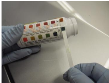
FIGURE 7-10 A test strip can be used to determine the pH and percentage of glycol of the coolant. The percentage of glycol determines the freezing and boiling temperatures, as shown on the bottle that contains the test strips.
