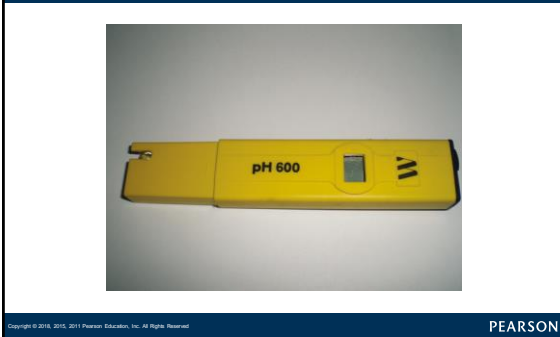
FIGURE 7-8 A meter that measures the actual pH of the coolant can be used for all coolants, unlike many test strips that cannot be used to test the pH of red or orange coolants.
