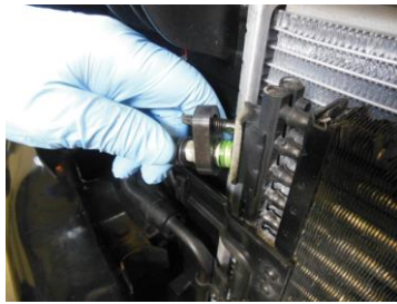
FIGURE 5-36 The line to the condenser from the compressor includes a flange mount with an O-ring. This line is being replaced with a new original equipment line as a result of an accident, which caused the line to be kinked.
