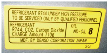
FIGURE 4-10 The label on a Toyota Fuel Cell Hybrid Vehicle (FCHV) showing that CO 2 (R744) is being used as the refrigerant.
