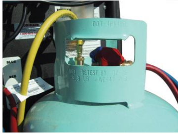
FIGURE 4-2 The stamped text at the top of this container reads "DOT-4BA400."
